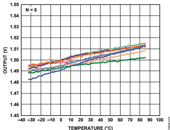
Figure 13. Y-Axis Zero g Bias vs. Temperature—
