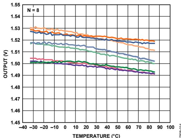
Figure 12. X-Axis Zero g Bias vs. Temperature—
