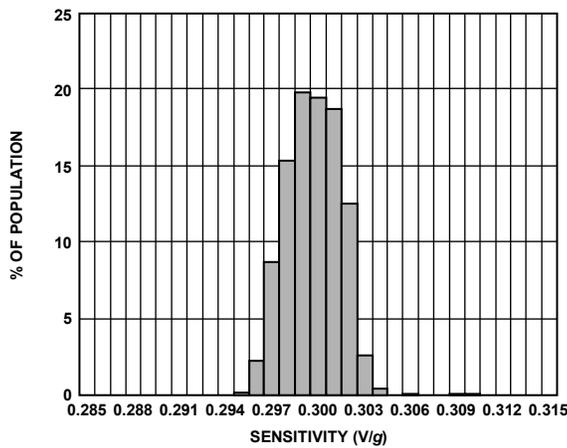
Figure 17. Z-Axis Sensitivity at 25°C,  $V_S = 3\text{ V}$
