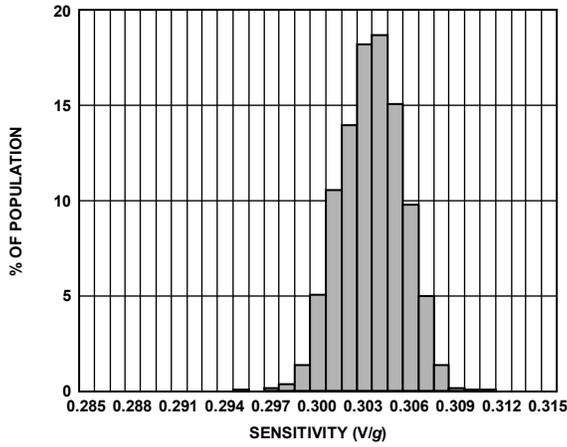
Figure 15. X-Axis Sensitivity at 25°C,  $V_S = 3\text{ V}$
