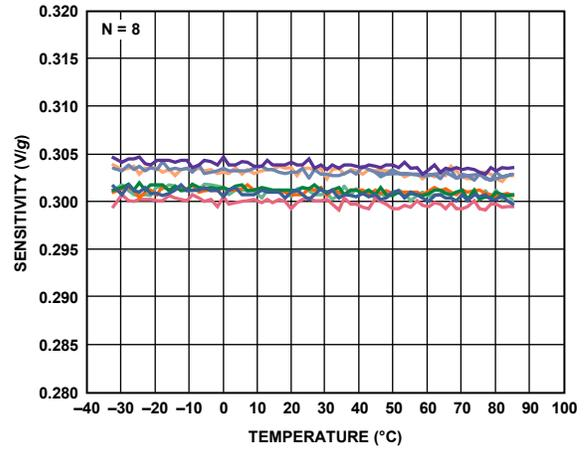
Figure 18. X-Axis Sensitivity vs. Temperature—
