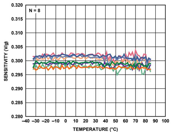
Figure 20. Z-Axis Sensitivity vs. Temperature—
