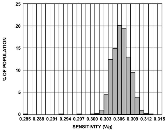
Figure 16. Y-Axis Sensitivity at 25°C,  $V_S = 3\text{ V}$
