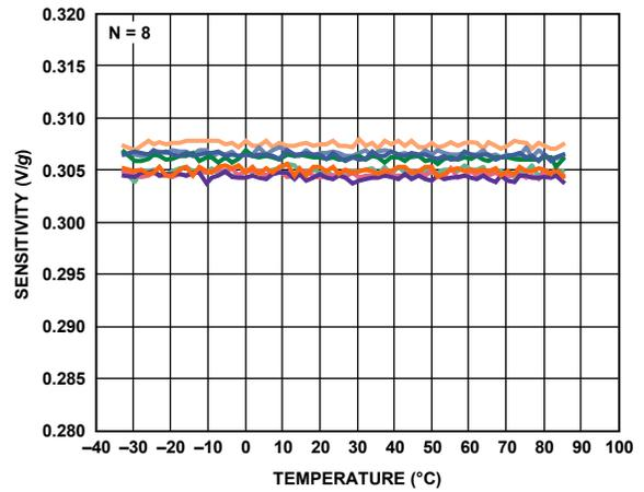
Figure 19. Y-Axis Sensitivity vs. Temperature—
